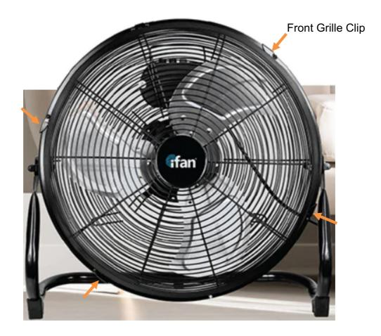
3. Clean the exterior parts of the fan (Front Grille, Back Grille, Fan Blade, Tube Base, etc.) thoroughly with warm water & dish-washing agent and a damp cloth, and immediately wipe dry. Make sure that the Motor Unit DOES NOT come into contact with water.
